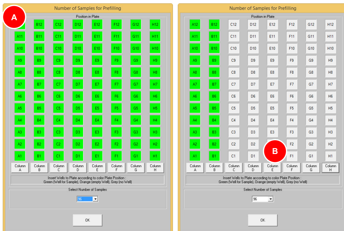
Fig. 29 Setting up the chemagic Dispenser for the chemagic 96 Rod Head
